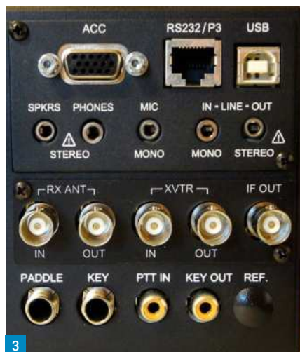
Fig. 1: The Signalink USB is a popular interface between computers and transceivers. Fig. 2: RTTY messages can become corrupted due to QRM, QRN and QSB. Fig. 3: The Elecraft K3S transceiver includes a built-in sound card. It can be connected to a computer simply with just a USB lead plugged into the rear panel shown here. Fig. 4: An FT4 contact with Thailand on 20m using just 10 Watts to a dipole antenna at about 6m above ground level. Fig. 5: An SSTV picture received from the International Space Station (ISS). Fig. 6: The Full Licence Manual is essential reading for those studying for their Full Licence exam. Fig. 7: The Exam Secrets book contains some additional material for all three exams as well mock exam questions.
